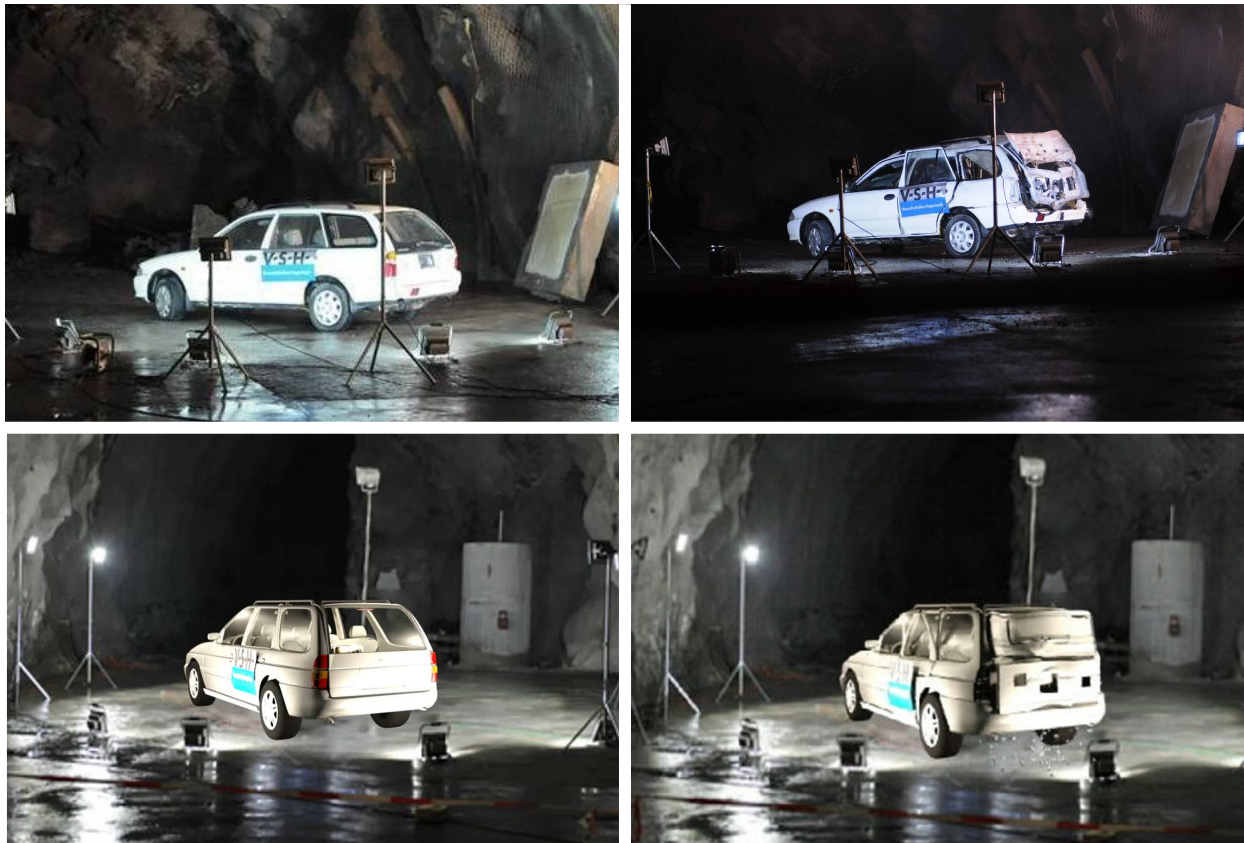
Photos above: Actual vehicle before and after the explosion. Photo courtesy: Max Wietek. Images below: Simulated vehicle before and after the explosion in 3ds-MAX.
