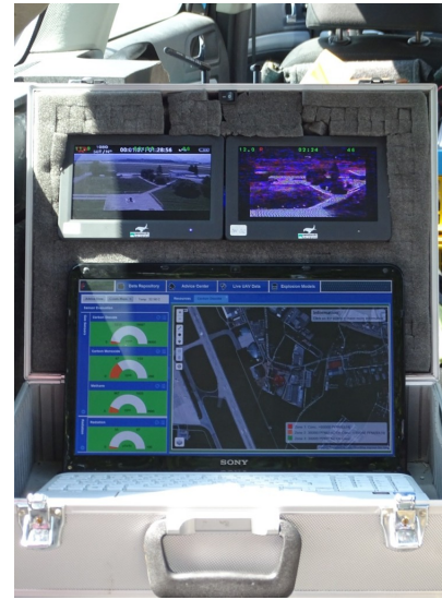
Ground-station with infrared and video images, and Expert System display.
