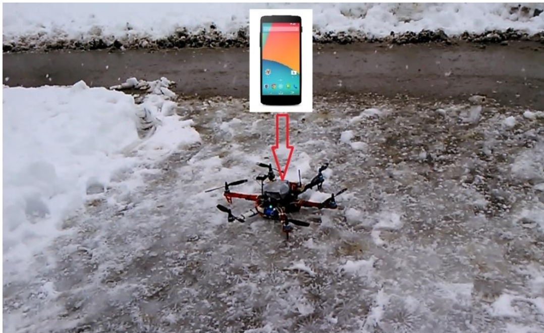
Figure 23 Field test of FIT Help Beacons system installed onboard of PLUS UAV Mk III.
