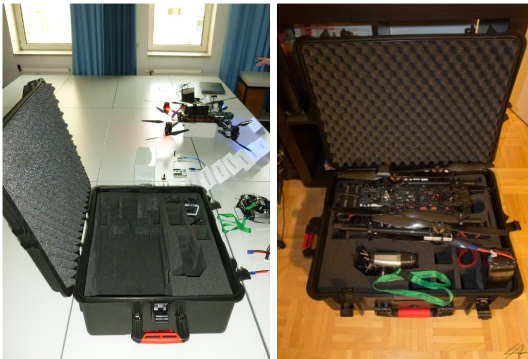
Figure 6 Water-protected, ruggedized transport case of complete PLUS UAV Mk III system with foldable arms.
