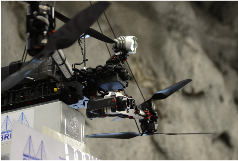
PLUS dual-quadcopter with video and infrared cameras, and a sensor box. Photo courtesy: Alexander Boden (Fraunhofer FIT).
