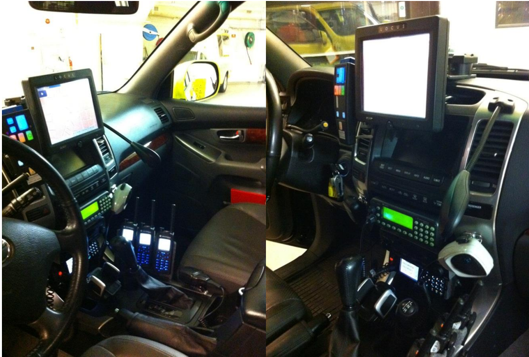
Figure 3. Locus TransMobile PC installed in a Norwegian ambulance vehicle.
